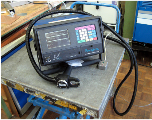
Figure 48. Swagelok orbital welding machine
